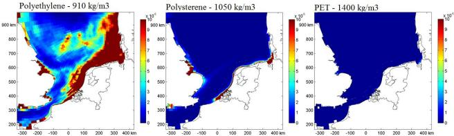
Figure 3. Mean concentration of particles in the water surface, calculated in last day of a simulation run of year 2008. Model simulations comparison of different plastic types (polyethylene, polystyrene, PET), spherical shape, diameter ~ 330 µm
